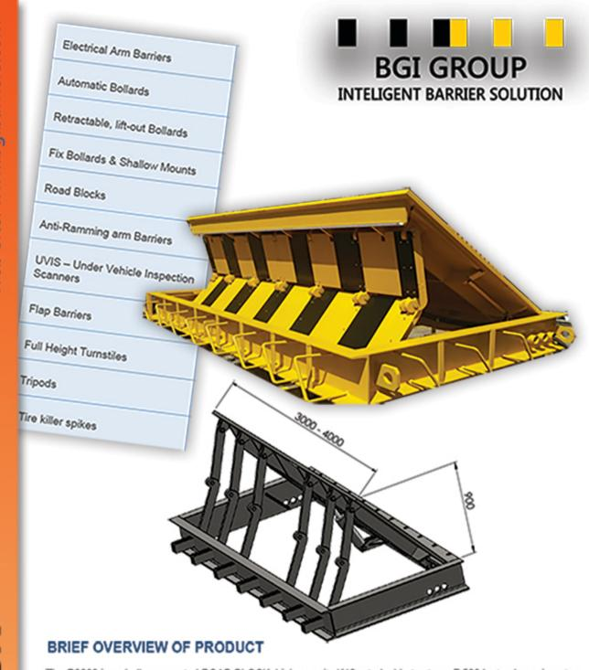
The R3000 is a shallow mounted ROAD BLOCK, high security K12 rated, able to stop a 7,500 kg truck moving at a speed of 80 kph. This product must be installed within an approved reinforced concrete foundation.
